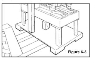
Transport the machine with a fork-lift truck to the operating position. Lift the pallet at the point indicated in **Figure 6-3** (weight of machine + pallet = See Specifications).
