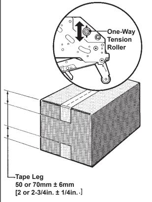
Figure 5-6 - Leading Tape Leg Length
