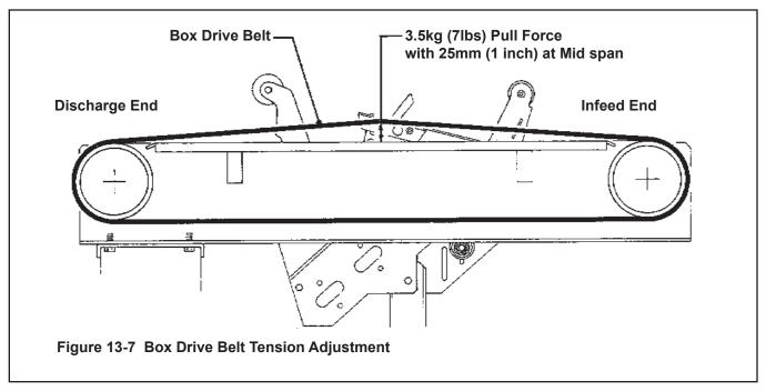
Refer to Figure 13-8 and 13-9 and adjust belt tension as follows:
