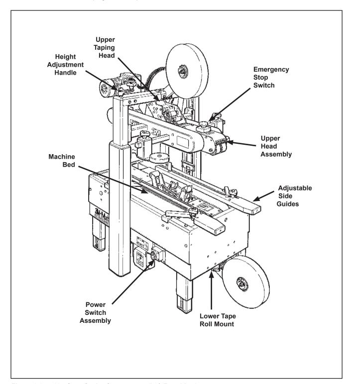
Figure 3-9—700a Case Sealer Components (Left Front View)
