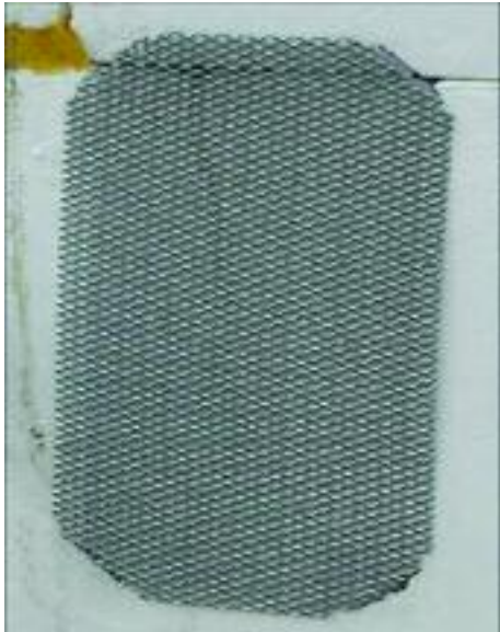
Fig 3.10 – Perforated steel backing plate (Grappler).
