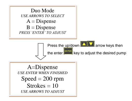
Speed can be adjusted based on the control type selected from the Input Setup section in the manual. By default the PDS-100 is configured for Keypad Control and Keypad Start.
