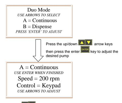
To adjust the speed press the up/down arrow keys until the desired speed is set. Notice how the speed immediately begins to adjust. To save press the enter key. The unit returns to main screen
