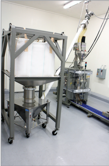
Hapman's Helix Flexible Screw Conveyor installed at the Guixens Food Group Facility in Tampa, Florida.
