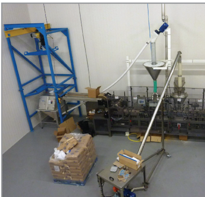
Hapman's Helix Flexible Screw Conveyor installed on a popcorn packaging line.
