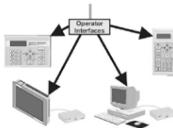
Figure T3 - VCM Controller Operator Interfaces
