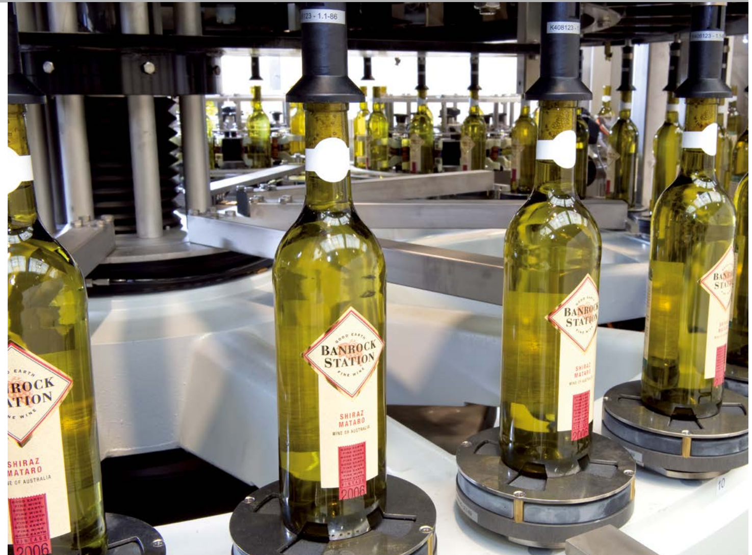
Servo-controlled container table in spoked wheel finish
