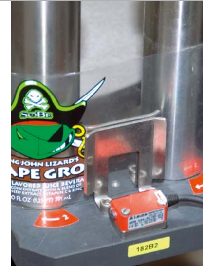
Precise recognition of the end of reel via sensor
