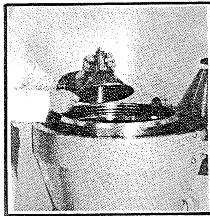
19 Lift out the distributing cone by hand (if it not had joined the distributor when the latter was lifted out). ⦿ Lock ring threads—p.3:3.
