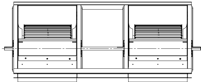
Typical Forward Curved Twin Fan Assy. for a Vertical Unit (Code 05= V) AND Top Horizontal Discharge (Code 23= TH)
