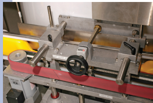
Quick size change using our hand wheel adjustment
