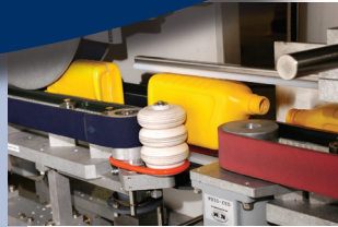
Gentle container handling w/ soft belt transfer system
