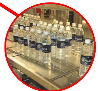
FLIGHT BARS LOAD PRODUCT (moving product across dead plate)
