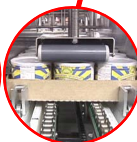
TOP COMPRESSION ROLLERS (as required)
