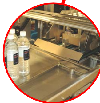
FLIGHT BARS LOAD PRODUCT (end of dead plate)
