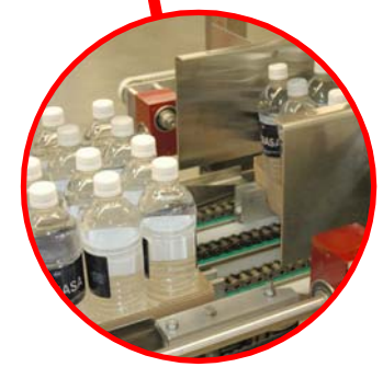
TRAYS ARE FORMED AROUND THE PRODUCTS
