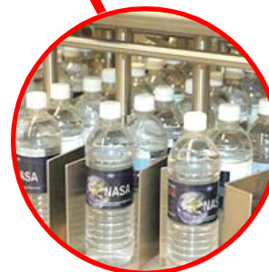
PRODUCT RELEASED FROM GATE (between flight bars)
