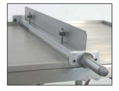
Adjustable Product Leveler: Set the desired depth and roll along side slab bars. It skims the top to a create an even batch
