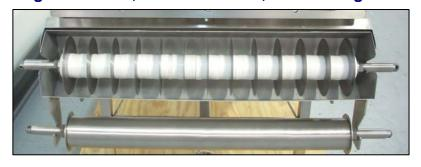
Rolling Drum Sizer Weighted drum to roll batch flat. Available in sizes to span width of table, or shorter lengths for smaller areas **<u>Table Cutter</u>** rolls along side slab bars and cuts entire length of batch. Side Saddles with Protective Cover for Table Cutter available Slab Bars Extra High or special sizes available as special order
