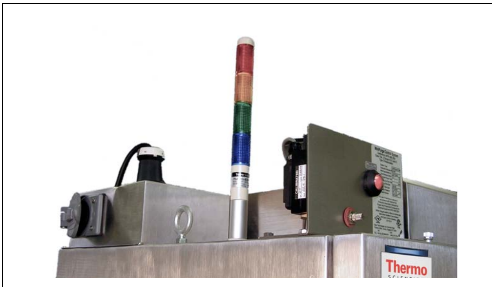
Figure C-20. Tower Light Installed
