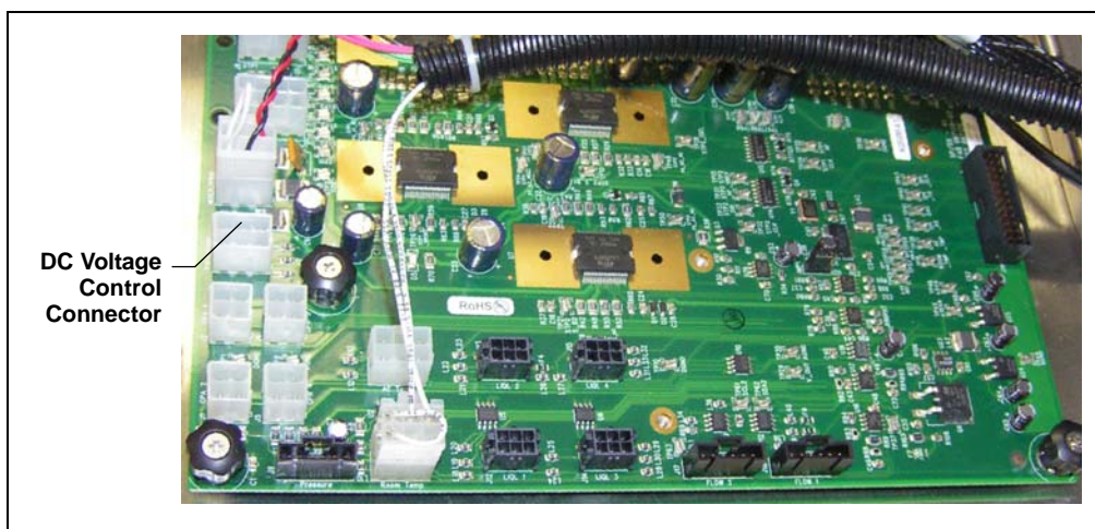
Figure 3-45. SP Electronics Board: DC Voltage Control Connector
