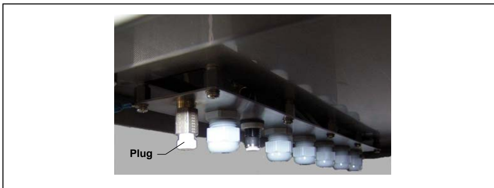
Figure D-14. Plug in AE Drain (Under the AE on the Left Side)
