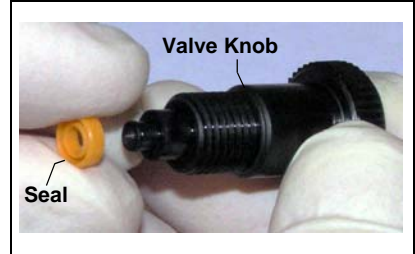
Figure 10-6. Waste Valve Seal Replacement
