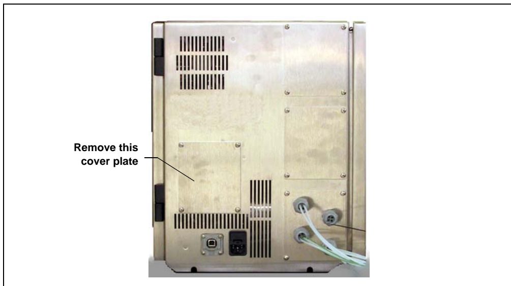
Figure C-3. Side of SP: TTL/Relay Panel Not Yet Installed
