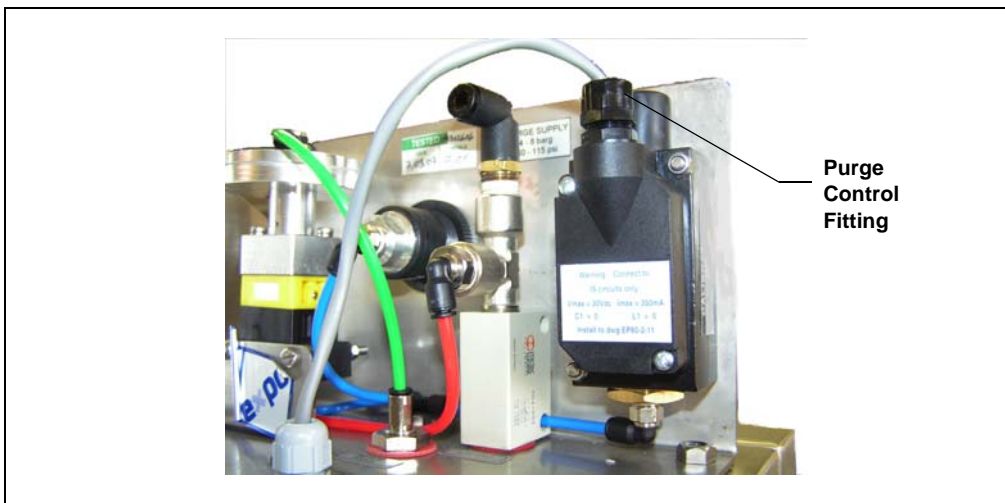
Figure D-7. Purge Control Unit Installed (Rear View)
