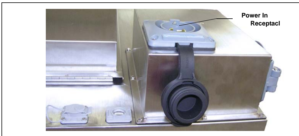
Figure 5-4. AE Power In Receptacle
