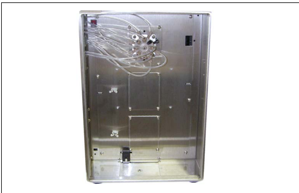
Figure 4-1. SS Stream Selector with One Stream Selection Valve
