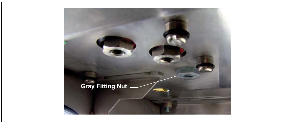
Figure D-2. AE Interior: Gray Fitting Nut Installed
