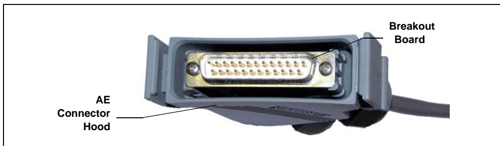
Figure C-14. Breakout Board Installed in the AE Connector Hood
