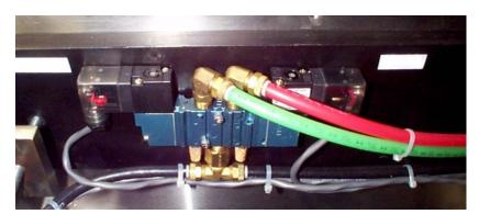
Figure 2-7: Double Solenoid Valve
